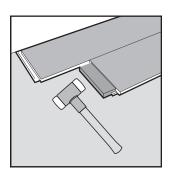
Use a tapping block and position it against the locking system. Gently tap the block with a hammer to gradually connect the panels in a few taps.
