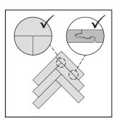
After installing a panel, check all joints to see if they are fully connected and there are no gaps or height differences.
