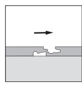
For areas where it is not possible to use angling or a tapping block, such as the end panels against the wall, use the pull bar. Start when the panels are flat on the floor.
