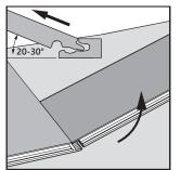
Angle up the end of the panel to angle out the short side. **UNILIN ANGLE-ANGLE / HERRINGBONE**
