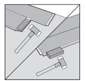
To ensure all gaps are closed, gently tap the tapping block with a hammer to completely close the joints.
