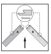
Lay down the panels in the correct start position with the groove side pointing away from the starter wall and to the outside of the V.
