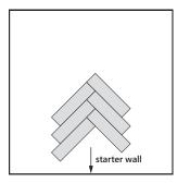
After a few panels, slide the row towards the starter wall, aligned with the center line of the room. Leave enough room for the expansion gaps.
