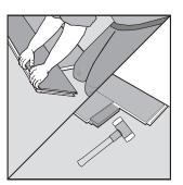
To install the next row, always connect the long side of the new panel into the installed panels.
