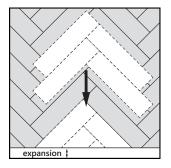
Pre-build the edge pieces with enough panels to cover the gaps. Measure the edges of the remaining floor, taking the expansion gap into account.
