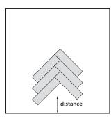
Start the installation at a distance away from the starter wall for easier installation.
