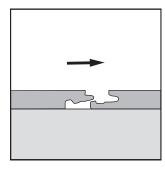
For locking in two sides or if angling is not possible, use the tapping method. If possible, angle in one side of the panel. Tapping is possible on the long and short side.
