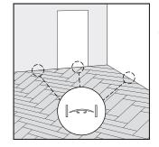
Provide expansion joints between different rooms or in large rooms. Check the supplier's guidelines for details.
