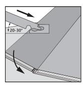
Start by locking in the long side. Position the panel at an angle of 20-30° to the panel that is already installed.
