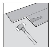
Place the pull bar against the panel. Gently tap the pull bar with a hammer to gradually connect the panels in a few taps.
